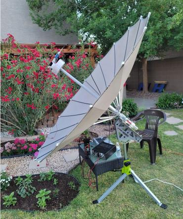
The SLS-FD6 is a lightweight 2.4m folding fabric parabolic dish with an integrated patch feed. The FD6 weighs just 10 lbs. and folds down to 8" x 8" x 54" for transport and storage. The integrated patch feed can remain in the dish when folded.
